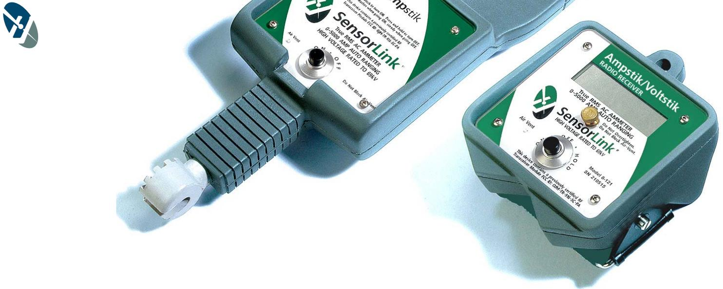
**The Radio Ampstik** uses the same current sensor technology as the original Ampstik. The key feature of this unit is the ability to display the current reading up to 50 feet away from the sensor. The user has the option to hold the display in their hands, mount it to a hotstick, or hang it on the bucket.
