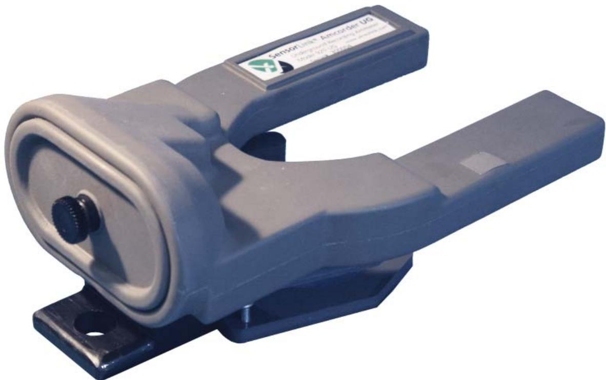
The **Amcorder UG** uses the same sensor technology and topology as the SensorLink® Ampstik®. The True RMS inductive sensor does not use magnetic materials and has no moving parts. The opening of the sensor is electronically closed and external currents are electronically rejected. The accuracy, external current reject, and range of currents measured by the patented amp sensor substantially exceed the performance of the best clamp-on sensors.
