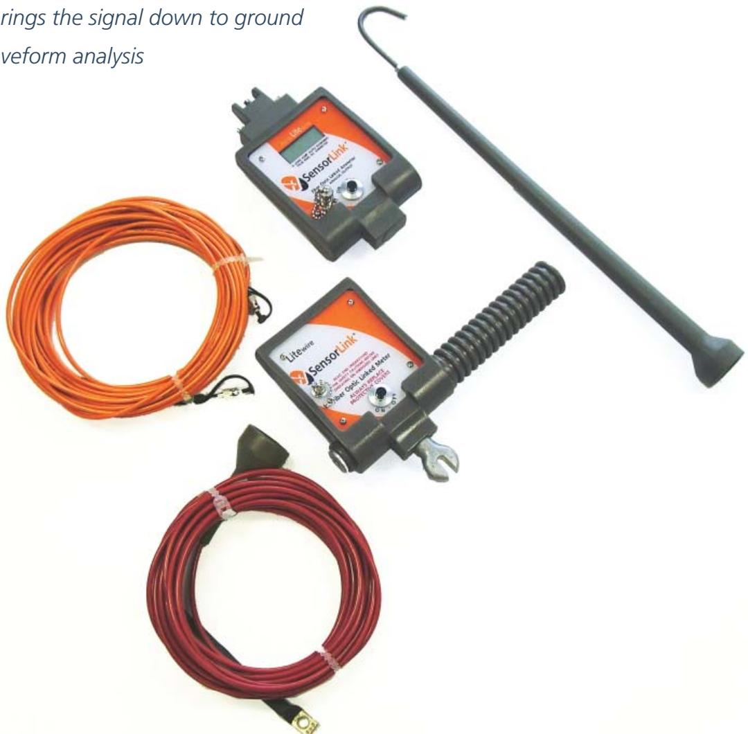
The Volt LiteWire is a medium voltage voltmeter designed for lines and substations. These units are designed for use with a hotstick and universal chuck adapter. The Volt LiteWire measures voltage phase to phase or phase to ground. It is a two-piece, True RMS voltmeter with a fiber optic link between the high voltage sensor and the readout at ground potential. The sensor is mounted on a hotstick and slipped onto a medium voltage line.
